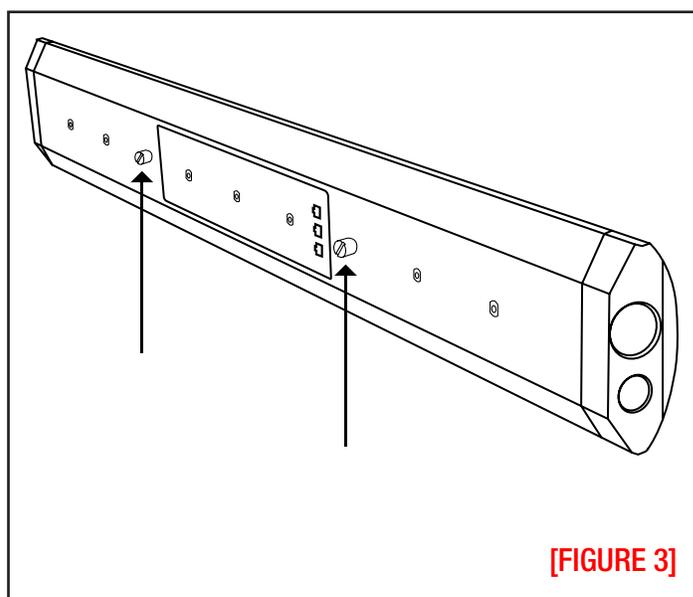
See step 3 for more detailed information on wiring the TSB3.0. Gently slide the Mounting Pins into the vertical mounting slots on the Mounting Brackets. Removal of the flat panel display may be necessary before mounting the TSB3.0. The Leveling Screws may be inserted in the bottom of the Mounting Bracket and used to adjust the height and to make sure the TSB3.0 speaker is level. Tightening the screw will raise the speaker and loosening it will lower it.
